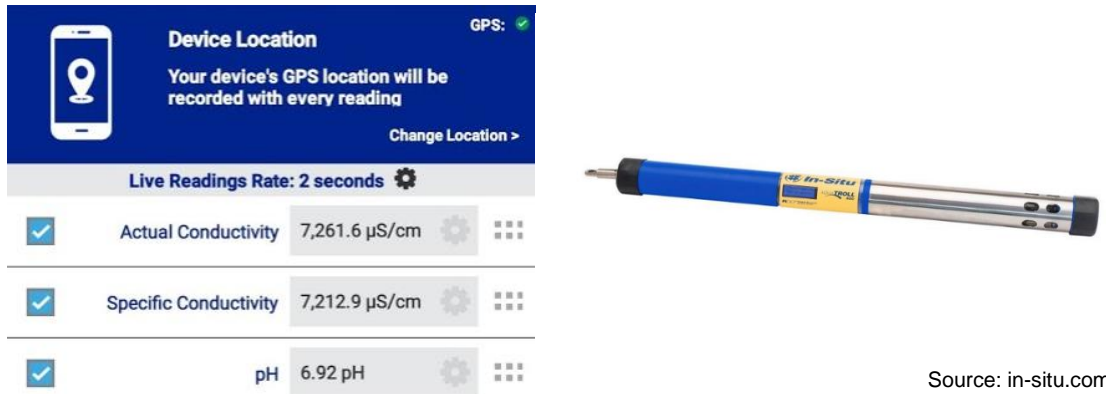
Figure A.4: Example of live readouts (left) being obtained from an Aqua TROLL 600 (right)
