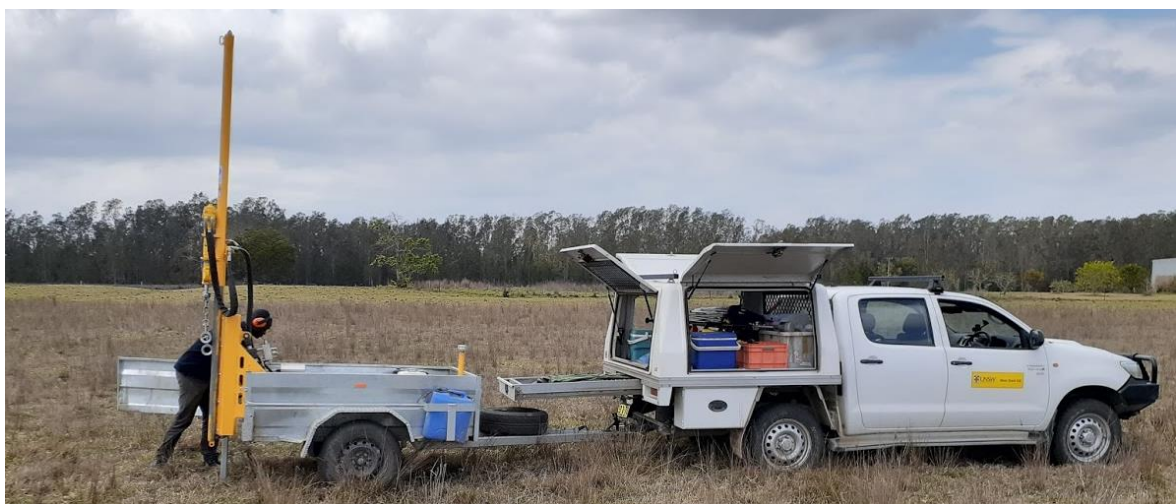
Figure A.5: The trailer mounted soil sampler being prepared for sampling
