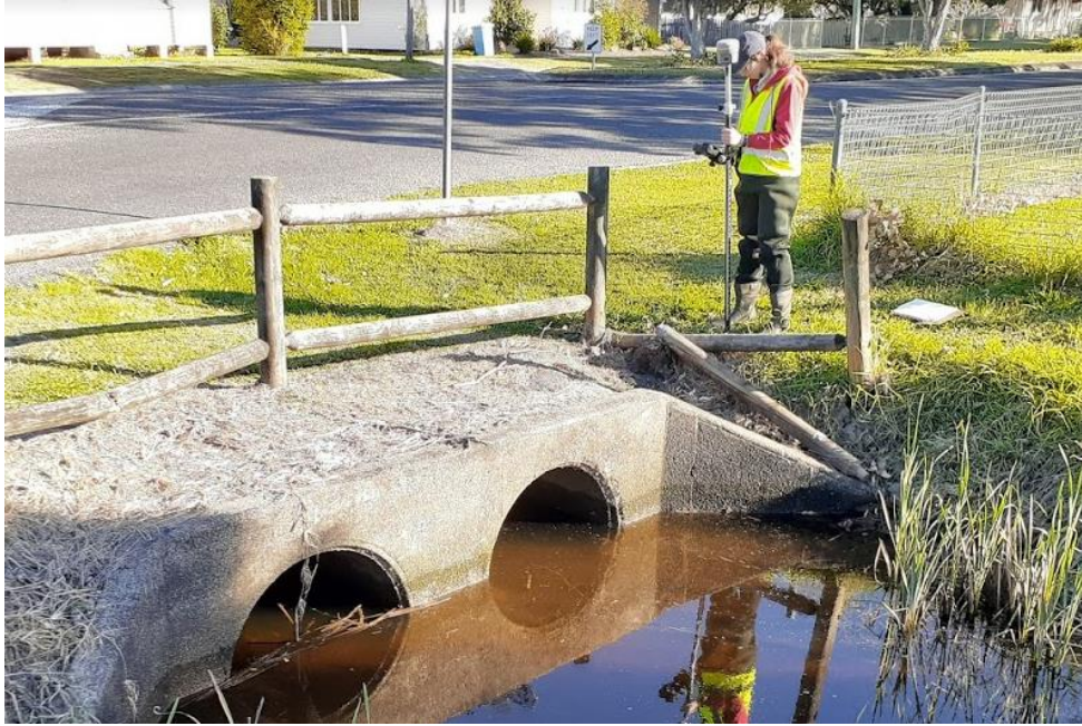
Figure A.1: A Trimble R10 GNSS receiver being used to survey culverts
