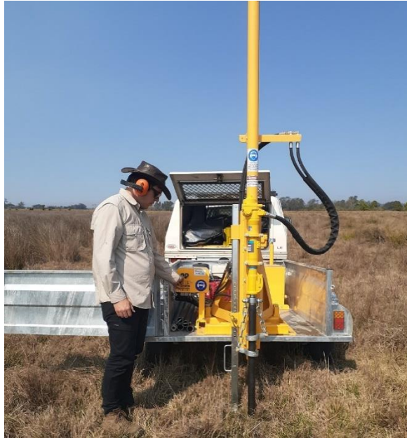
Figure A.6: The trailer mounted soil sampler being used to push a 51 mm hollow flight push tube into the ground to collect a soil profile
