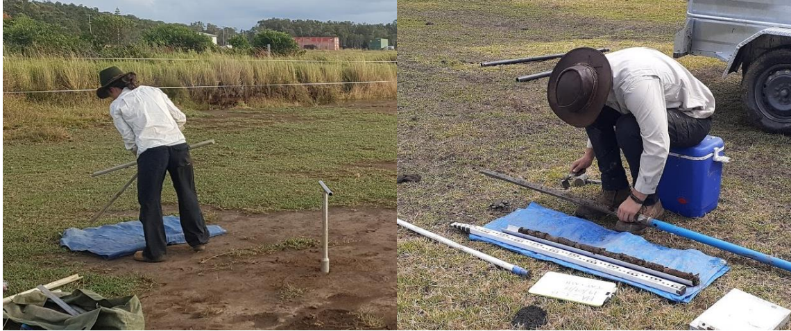
Figure A.8: A soil auger (left) and gouge auger (right) being used to collect soil samples
