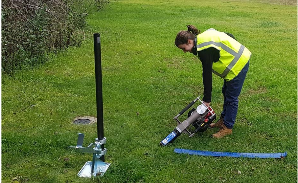
Figure A.7: Post hole driver soil sampler with manual foot pedal tube extractor
