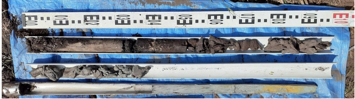
Figure A.9: Example of a soil profile laid out to have the properties of each layer recorded and analysed
