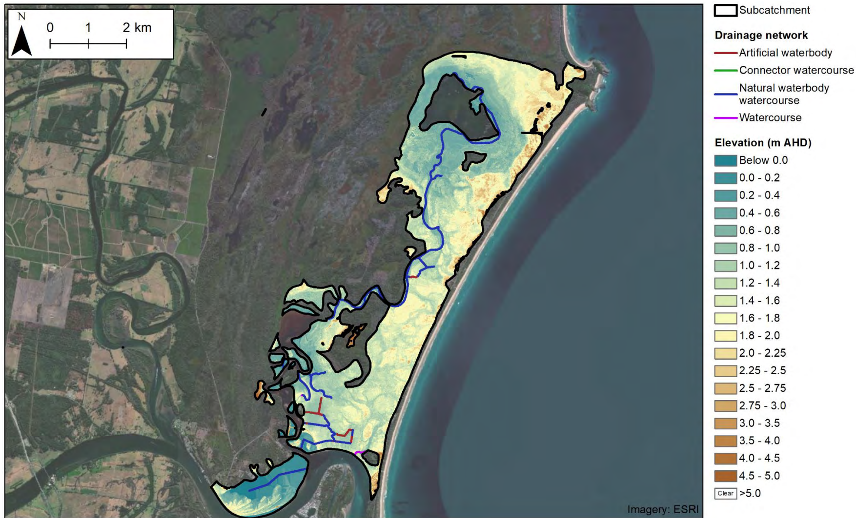
Figure 8-70: Limeburners Creek subcatchment elevation and drainage network
