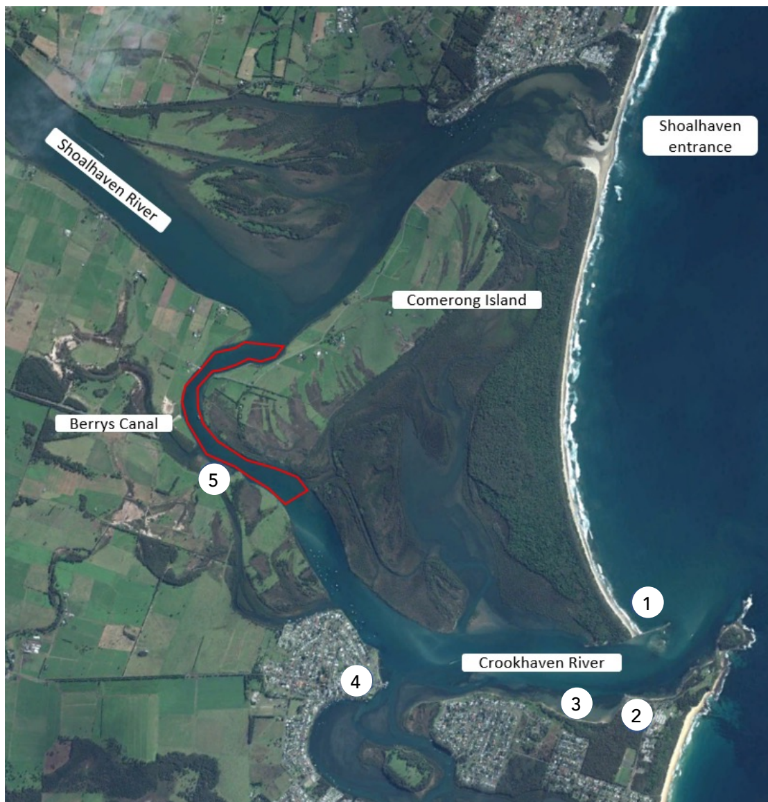
The Shoalhaven – Crookhaven estuaries are artificially linked by Berrys Canal shown in red and: (1) Crookhaven breakwater; (2) Crookhaven Regional Boat ramp breakwater; (3) First Street training wall; (4) Greenwell Point; (5) Numbaa training wall Credit: Google Earth
