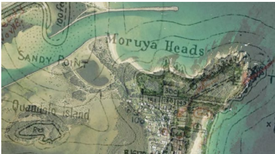
left: A 1917 Parish Map over a contemporary aerial photo shows the accretion of sand forming 320 m of ocean front sand beach south of the current southern breakwater
