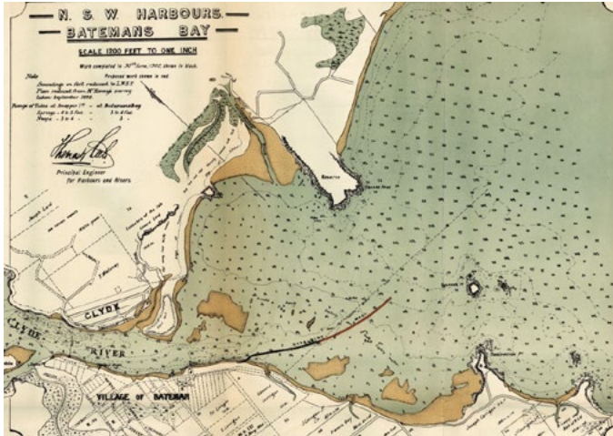
Chart showing progress on installing the southern training wall in 1902.
