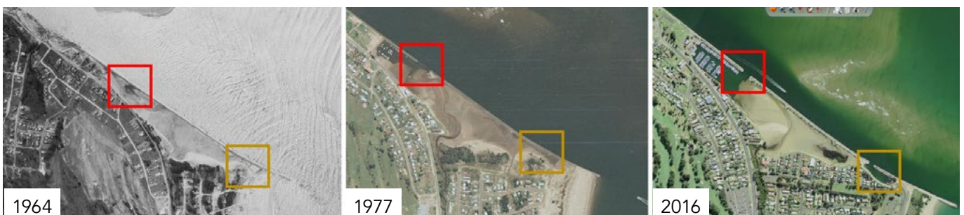
Progressive time series of aerial photos of the Clyde River estuary at Batemans Bay (left to right: 1964, 1977 and 2016). A break was made in the training wall to create the marina in 1978 and, later, another break created Hanging Rock boat harbour and the ramp at the eastern end
