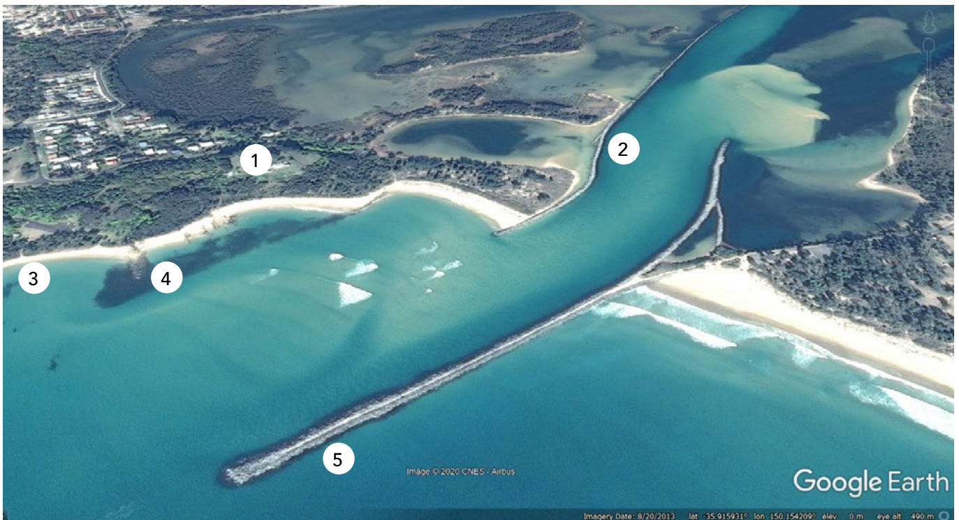
The Moruya River and its trained entrance: (1) the Meteorological Station; (2) end of the original southern training wall; (3) Shelly Beach; (4) abandoned southern breakwater; (5) northern breakwater. Source: Google Earth
