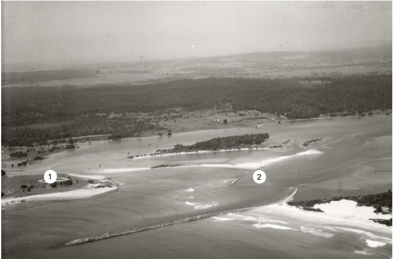
Aerial photo from November 1937 showing the trained entrance of Moruya River showing (1) the Meteorological Station and (2) the end of original southern training wall (also in the aerial photo below) Source: Adastra Aerial Photo Collection
