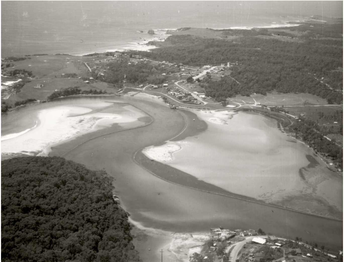
Aerial photo from November 1937 showing the trained entrance in the Wagonga River estuary. Further works, including construction of the breakwaters occurred in 1977–78 Source: Adastral Aerial Photo Collection
