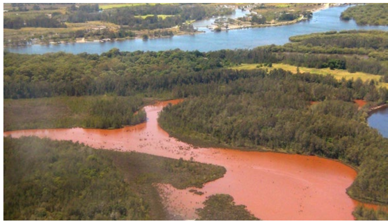
Yarrahapinni aerial iron stain, showing water behind the floodgates which is loaded with aluminium and heavy metals including arsenic from the acid sulfate soils (Mitchell Tulau/DPE)
