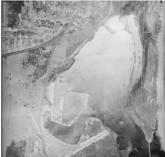
Aerial photo from 1951 (left) and 1990 (right) showing changes and the reclamation of Tom Thumb Lagoon with the construction of the coal loading wharf and other infrastructure in the inner Port Kembla Harbour area. The Tom Thumb Lagoon was described by George Bass and Matthew Flinders following a 1796 expedition undertaken in the 2.5 m open vessel called Tom Thumb II. Credit: Crown Lands
