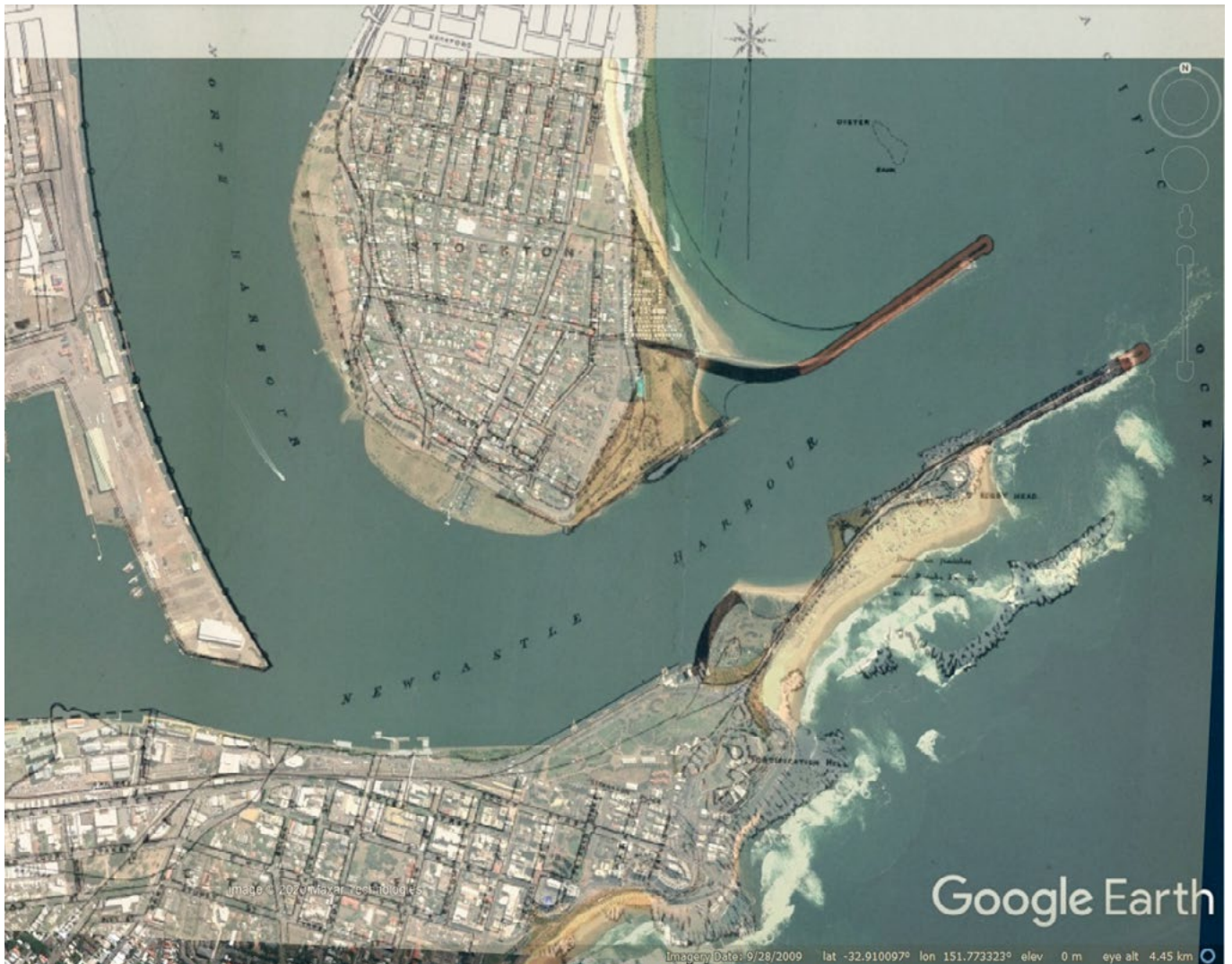
Changes in the shape of the Hunter River estuary and its trained entrance from 1902 to 2009 are shown by merging the above two images Credit: Google Earth
