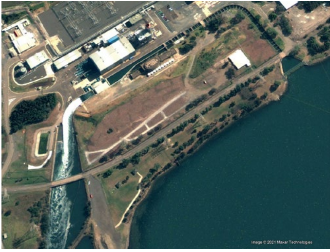
The discharging cooling water is channelled by the breakwater (LHS) which incorporates a boat ramp and a smooth crest surface that provides opportunities for all to walk along the breakwater Credit: Crown Lands and Google Earth
