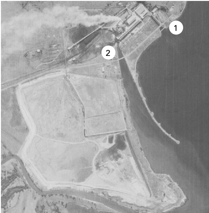
Tallawarra power plant and the Yallah Bay Breakwater showing: (1) the power plant water coolant inlet and (2) the outlet of the cooling water returning into Lake Illawarra in 1963 (left) and 2016 (right) Credit: Crown Lands and Google Earth
