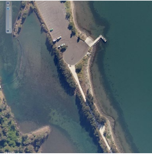
The discharging cooling water is channelled by the breakwater (LHS) which incorporates a boat ramp and a smooth crest surface that provides opportunities for all to walk along the breakwater Credit: Crown Lands and Google Earth
