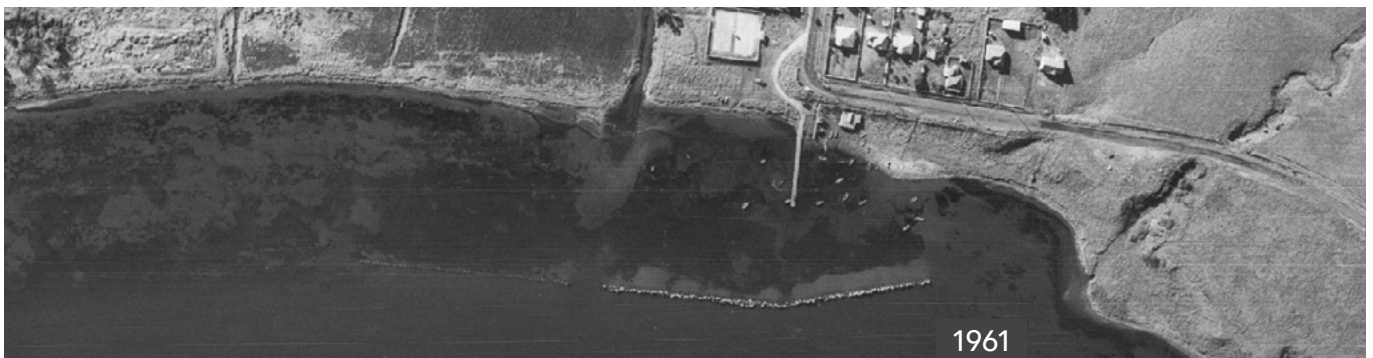
Berkeley Harbour began as a sheltered area behind a small offshore breakwater built from repurposed WWII tank traps Credit: Crown Lands
