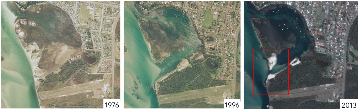
Aerial photo images of Swan Bay in 1976; in 1996 a large channel that formed in response to commercial dredging; and, after the channel was narrowed by installing two groynes Credit: Crown Lands
