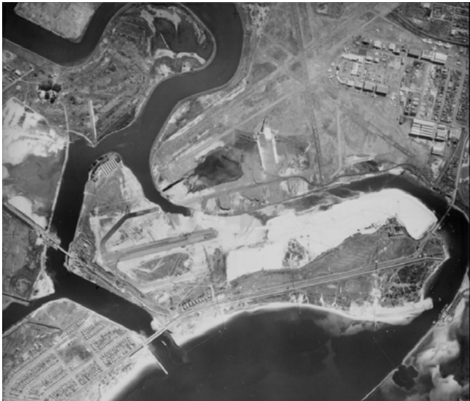
An aerial photo (left) and map (right), both from 1951, show airport reclamation works resulting in the diversion and training of the Cooks River entrance into Botany Bay Credit: Crown Lands
