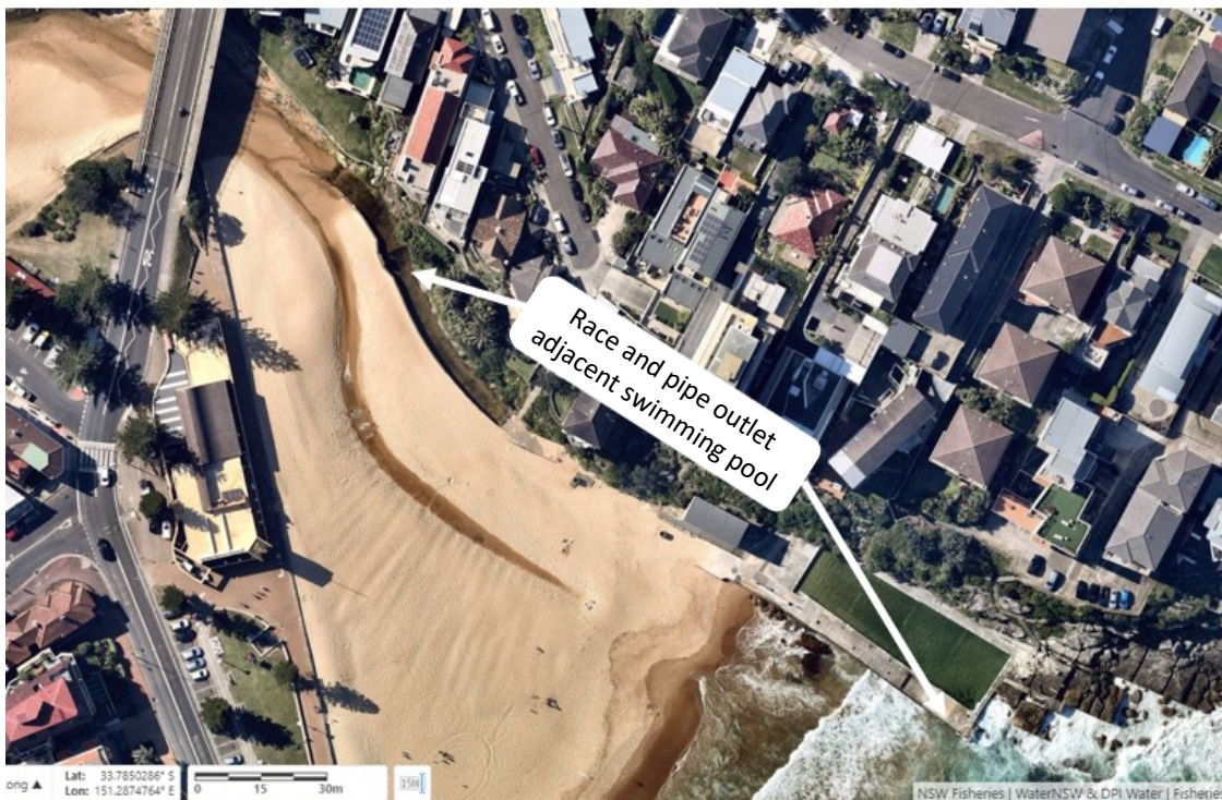
The Manly Lagoon estuary entrance was modified in the 1940s to incorporate a race and pipe outlet network. Source: nearmap and Crown Lands
