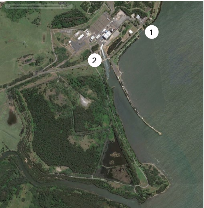
Tallawarra power plant and the Yallah Bay Breakwater showing: (1) the power plant water coolant inlet and (2) the outlet of the cooling water returning into Lake Illawarra in 1963 (left) and 2016 (right) Credit: Crown Lands and Google Earth
