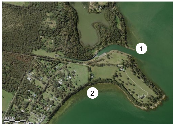
The Eraring Power Station coolant water is returned into Myuna Bay within Lake Macquarie via a constructed outlet (1) armoured with a breakwater. The location of the outlet is shown in 1976 (left) before it was constructed and in 2018 (right) Credit: Crown Lands and Google Earth
