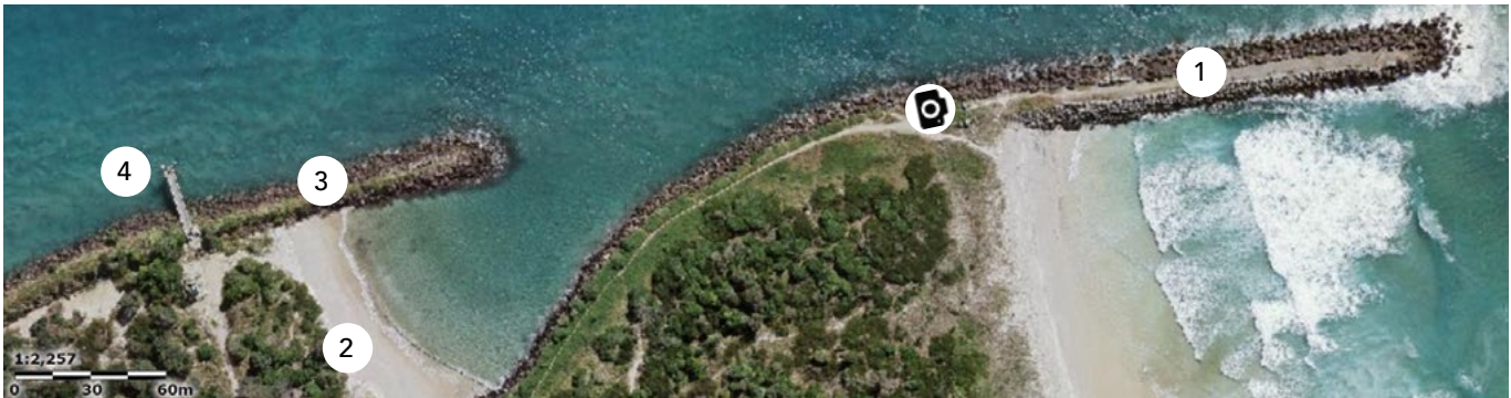
Southern Tweed River Breakwater: (1) the 1960s breakwater extension; (2) wave-trap beach; (3) original breakwater now part of estuarine training wall; (4) tidal gauge station and the water intake valve for the sand bypass scheme Credit: Six Maps
