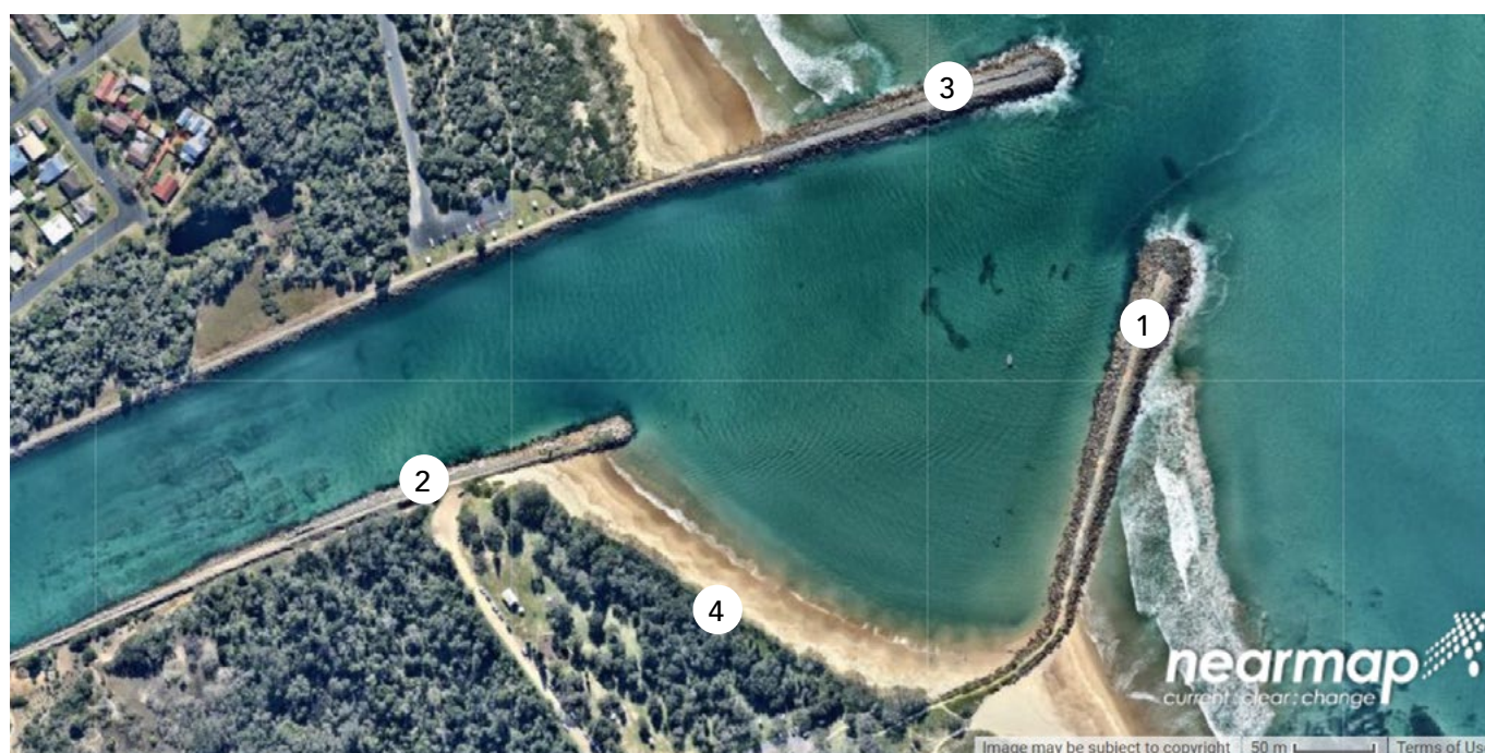
Aerial photo of the Camden Haven breakwaters: (1) new southern breakwater constructed in 1960s; (2) original southern breakwater; (3) northern breakwater; (4) Pilot Beach, a wave-trap beach reliant on the breakwater network
