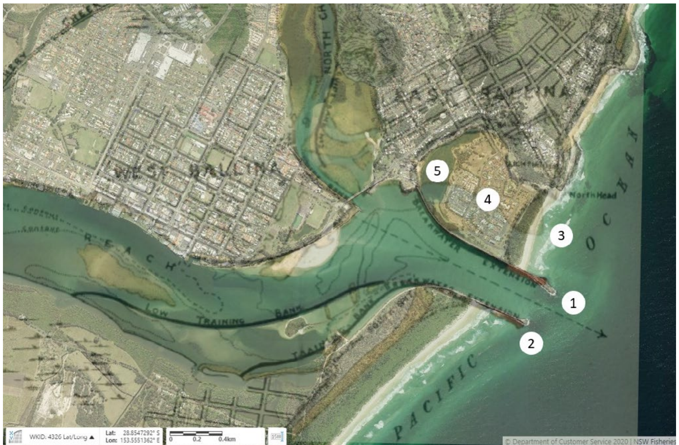
Changes in the shape of the Richmond River estuary due to the training walls are shown by merging the above two images, detailing: (1) northern breakwater; (2) southern breakwater; (3) Lighthouse Beach; (4) Shaws Bay urban development; (5) Shaws Bay sea lido; (6) Martin Street Boat Harbour; (7) Ballina Boat Harbour (approximately 300 m upstream).
