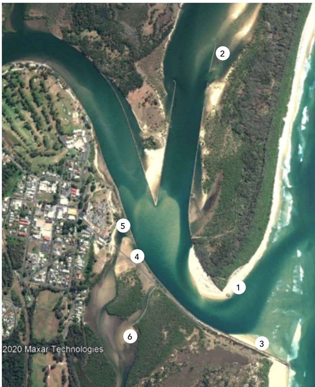
The Bellinger and Kalang Rivers estuary entrance showing (1) northern breakwater; (2) Bellinger River training wall; (3) southern breakwater; (4) Urunga pedestrian boardwalk; (5) Urunga sea lido; (6) Urunga Lagoon
