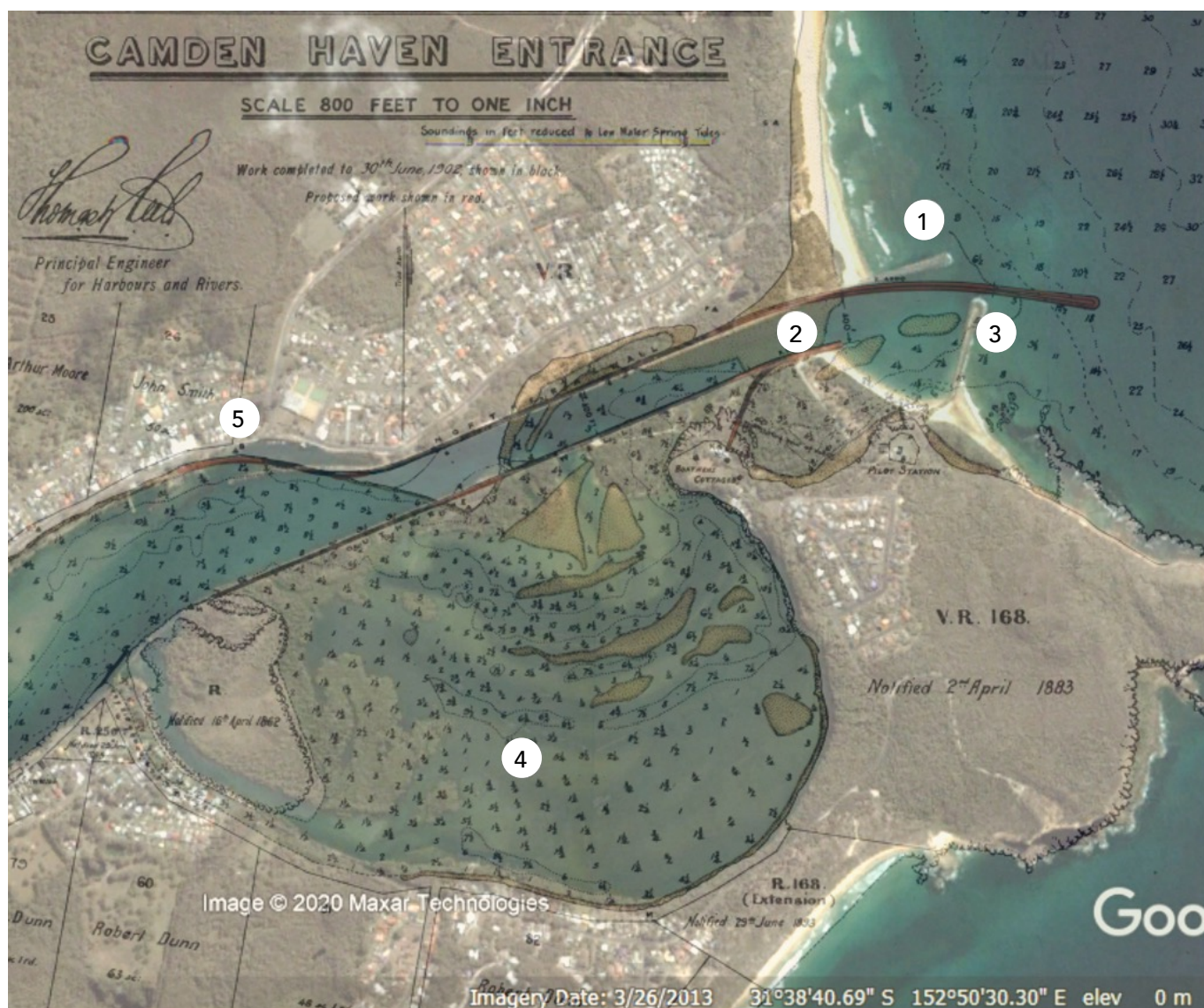
Changes in the shape of the Camden Haven River estuary due to the training walls are shown by merging the above two images detailing: (1) northern breakwater; (2) original southern breakwater; (3) new southern breakwater; (4) Gogleys Lagoon; (5) North Haven boat harbour precinct
