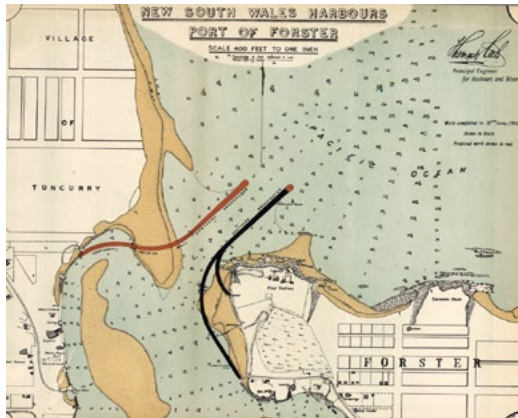
Chart showing progress on entrance training works at the Wallis Lake estuary entrance in 1902 Source: NSW Public Works Department 1902 Annual Report
