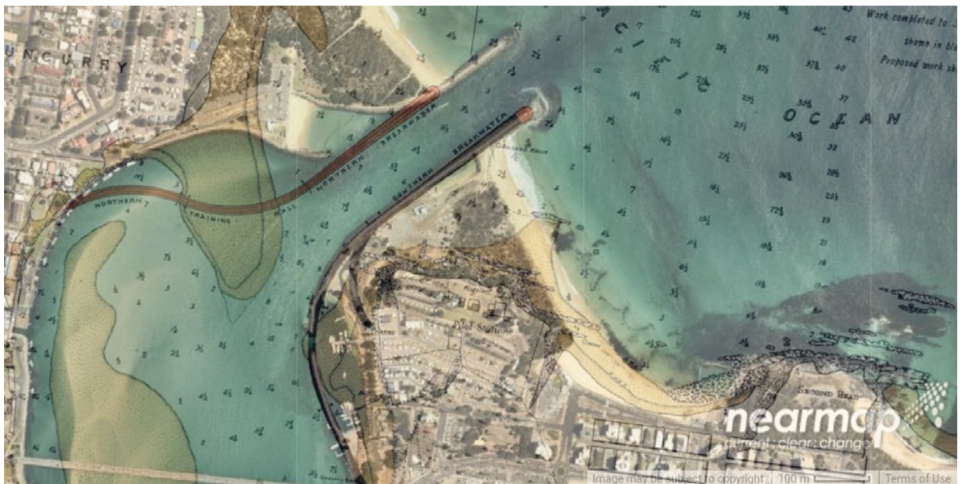
Changes in the shape of the Wallis Lake entrance and the adjacent ocean beaches due to the installation of training walls and breakwaters since 1902 are shown by merging the above two images.
