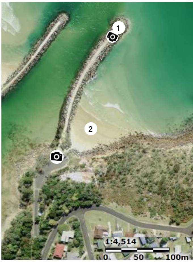
Evans River Breakwater with: (1) southern breakwater; (2) Shark Bay, a surf beach that was created when the breakwater was built. Credit: Six Maps
