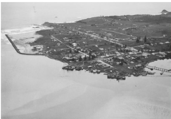
The 1933 aerial photograph from the Fairfax Collection (left) shows backwater areas behind the southern breakwater. These areas have progressively been reclaimed for a car park, playground facilities and caravan park (right)
