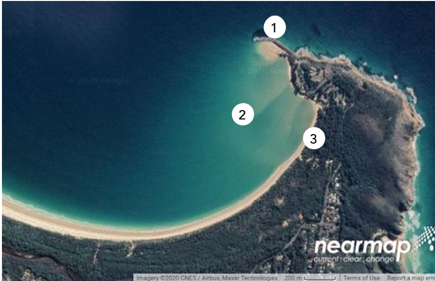
Trial Bay and South West Rocks in 2020 with (1) Laggars Point breakwater; (2) shoaling within Trial Bay; (3) accretion of sand and growth of vegetation advancing into Trial Bay Credit: nearmap
