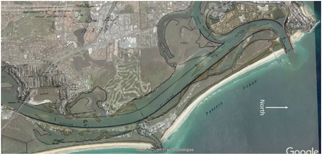
Changes in the shape of the Tweed River estuary due to the training walls from 1902 to 2017 are shown by merging the above two images
