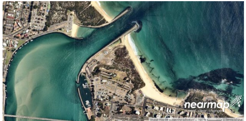
The entrance training at the entrance of Wallis Lake in 2020 Credit: nearmap
