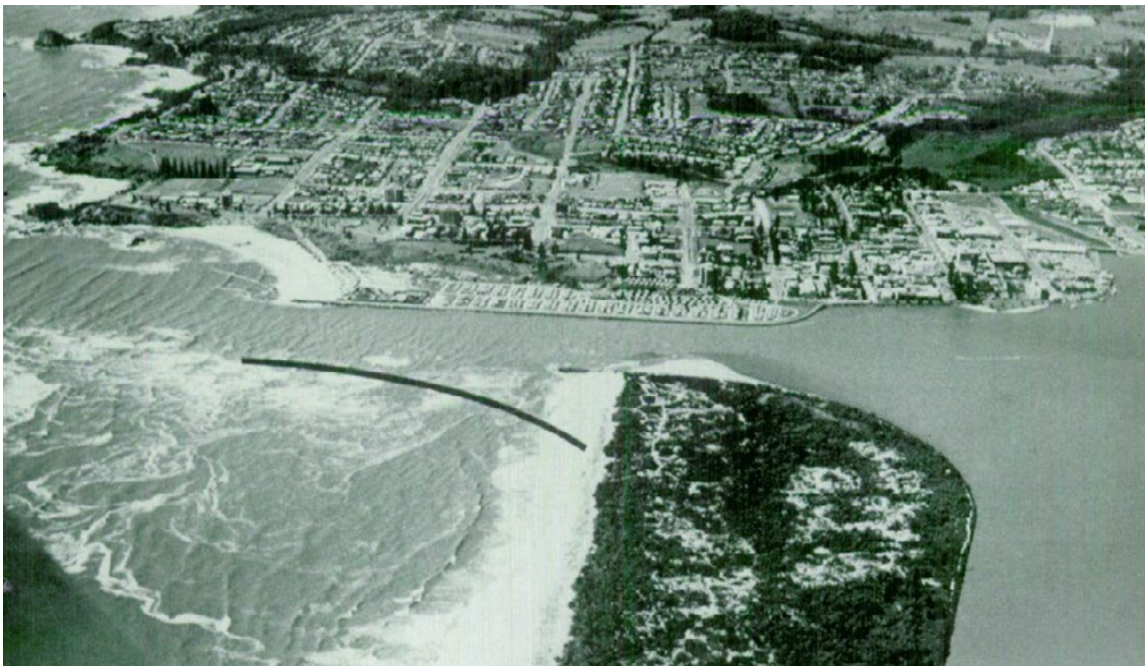
A 1977 aerial photo shows the approximate location of the then-proposed northern breakwater Source: NSW Public Works Department 1977 Annual Report
