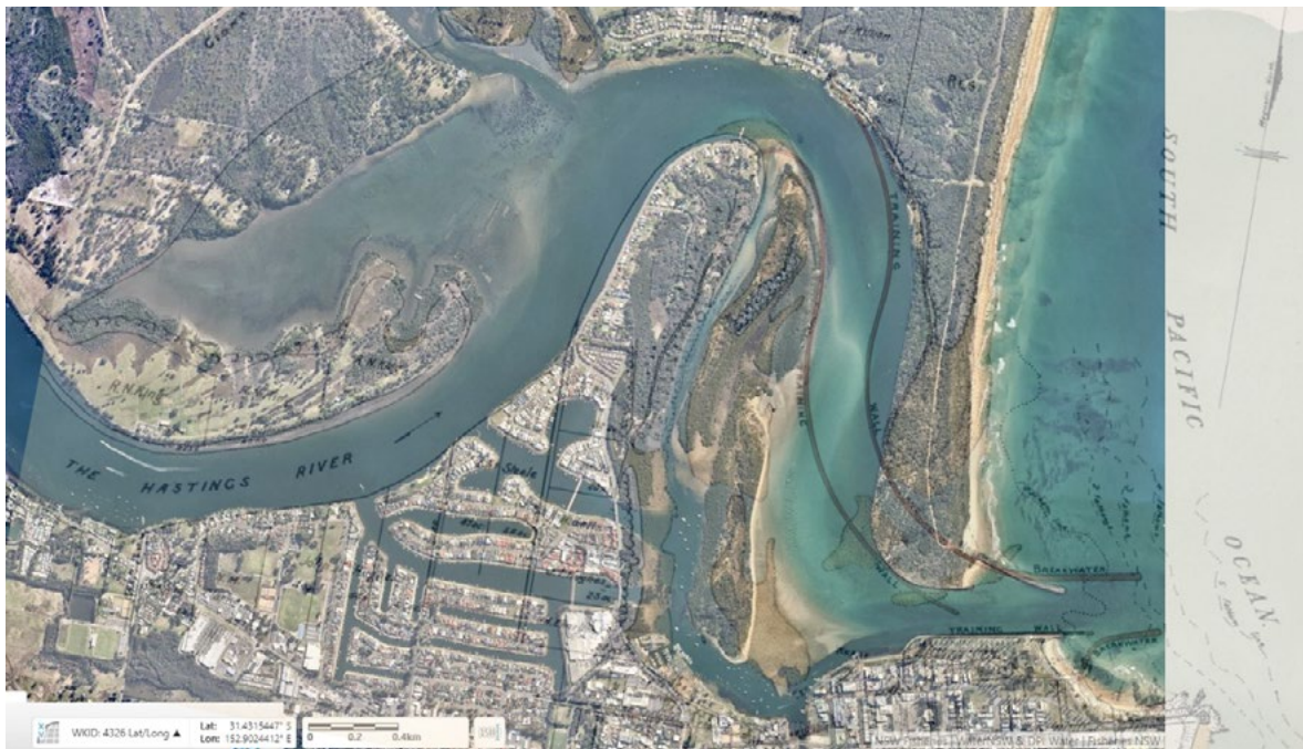
Changes in the shape of the Hastings River estuary since 1902 due to the training walls are shown by merging the above two images
