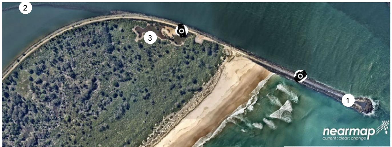
Aerial photo showing: (1) southern breakwater; (2) a half-tide training wall; (3) saltmarsh community reliant on tidal flushing through the breakwater Credit: nearmap
