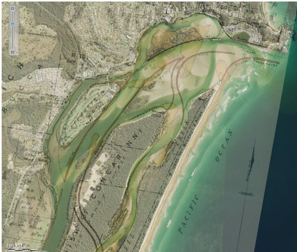
Changes in the shape of the Nambucca River estuary due to the training walls are shown by merging the above two images
