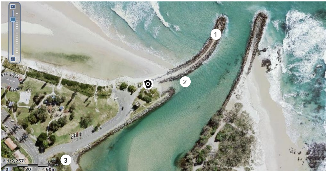
Cudgen Creek: (1) the northern breakwater; (2) wave-trap beach; (3) council boat ramp Credit: Six Maps
