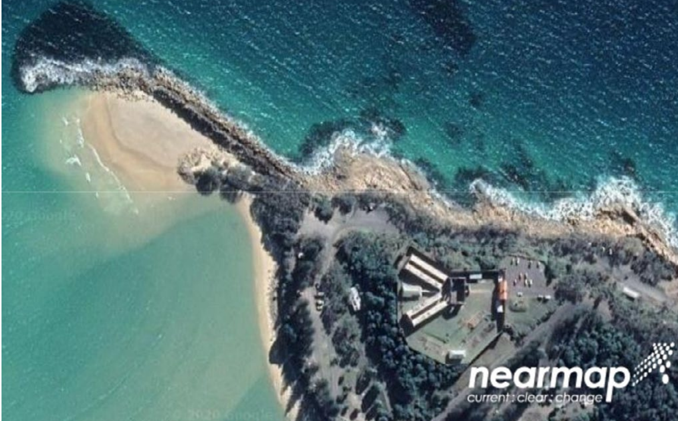
The breakwater was never completed and has resulted in accretion in Trial Bay Source: nearmap
