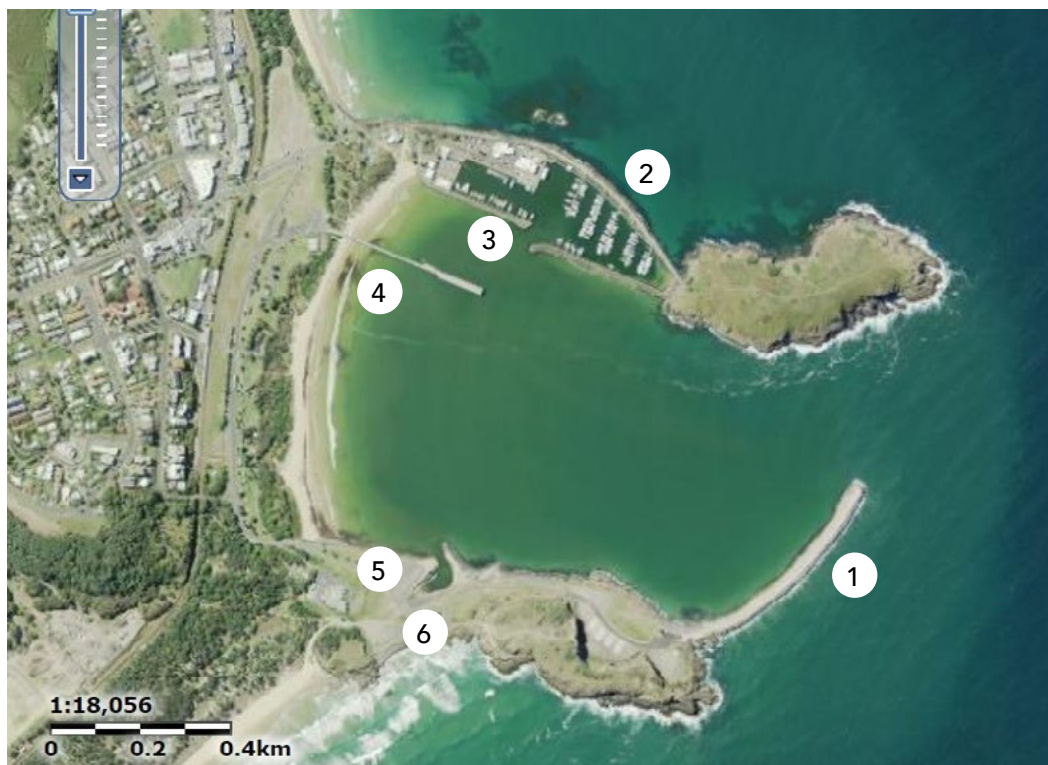
Coffs Harbour: (1) eastern breakwater; (2) northern breakwater; (3) inner breakwaters (east and west); (4) Coffs Harbour Jetty; (5) The Causeway, a reclaimed area joining the former South Coffs Island to the mainland and creates, (6) the 150 m long, southeast facing, Gallows Beach. Credit: Six Maps
