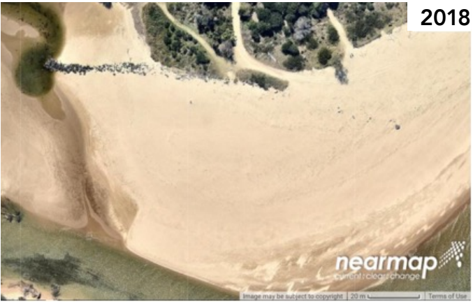
Shifting sands in Coffs Creek sometimes bury the northern training wall and expose it at other times.
