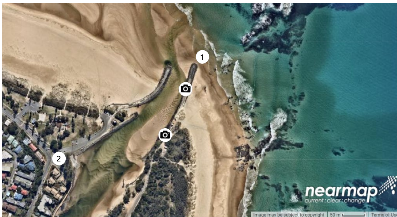
Cudgen Creek breakwater: (1) southern breakwater; (2) council boat ramp Credit: nearmap
